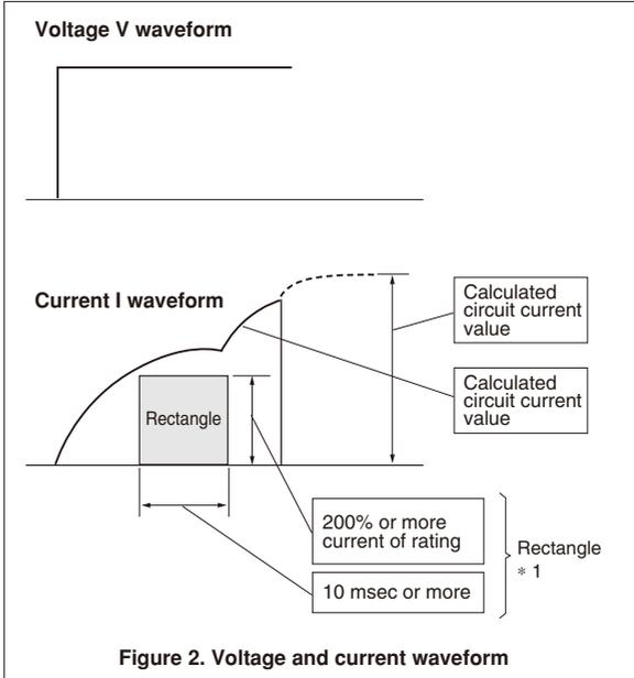
When high-speed operation is required (operation at 200% or more of rated current and minimum input pulse of 10 msec or less), please select a coil rating that can secure a rectangle\*1 within the actual circuit current waveform
