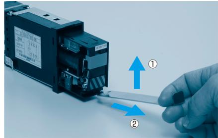
\* When removing the internal element, hang an element unplugging tool on the lower hook to unplug by lifting and removing the lock.
